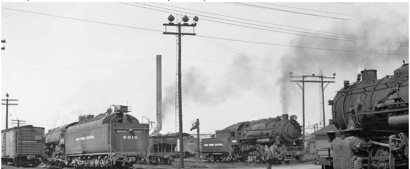
4-8-4 S-1b #6015, 0-8-0 U-3a #7816 and 2-8-2 H-7e #1995 all are at the Shelby Street Roundhouse just east of downtown Indianapolis during the twilight of steam in April 1956. Jermy Taylor Photo NYC SHS NG503044
