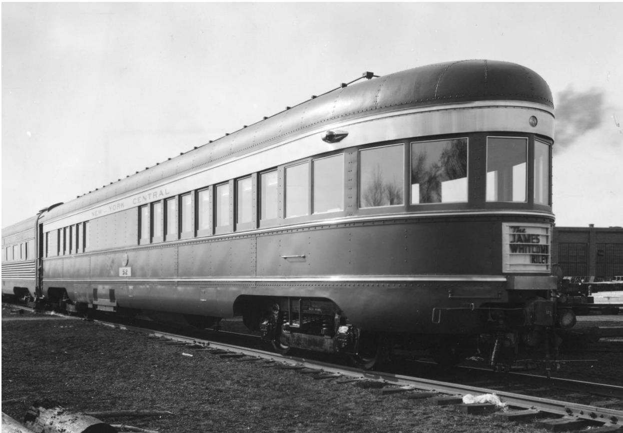
Bringing up the rear was lounge-observation #52. It was originally built by Pullman in 1927 as coach #746. It was rebuilt to observation-coach #52, then streamlined at Beech Grove in 1941.
