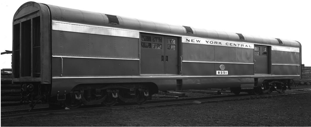
Baggage car 8551 was rebuilt at Beech Grove in 1941. It was originally built by American Car & Foundry in 1927 as NYC 3078 and renumbered c. 1935. NYCSHS WR280642
