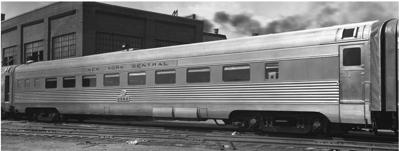
Coaches 2562 and 2563 built in 1939 and 1940 by Budd seating 60 in each car. NYCSHS WR280637 and WR280641
