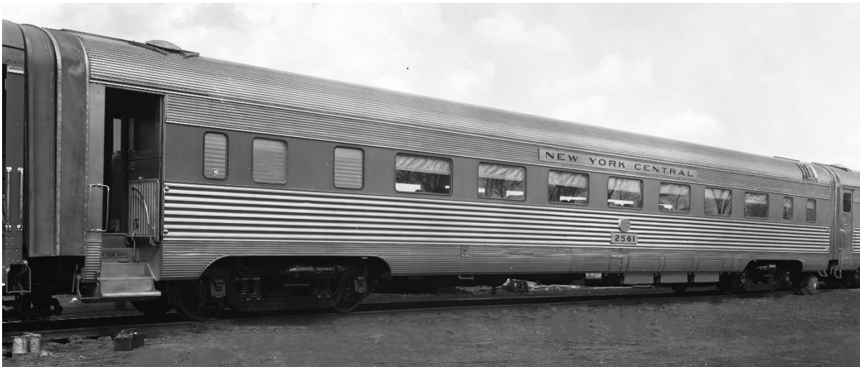
Coaches 2560 and 2561 were both 1938 products from Budd seating 52 each. NYCSHS WR280640 and WR280639
