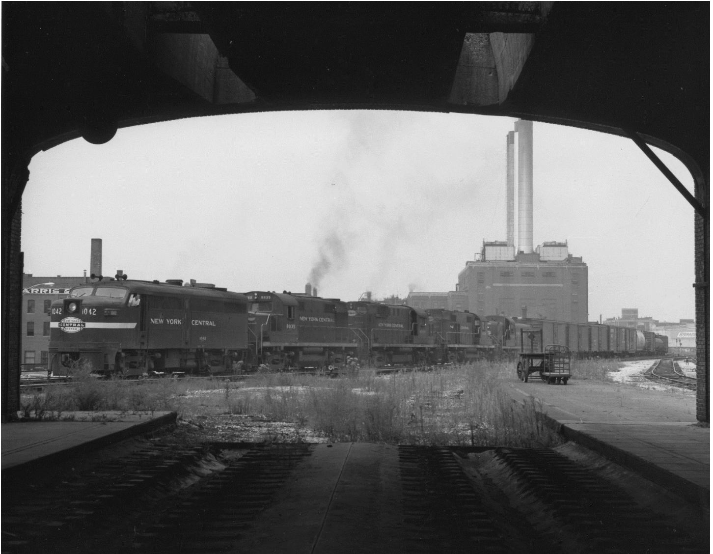
DFA-3e 1042 (Alco FA-1), DRS-12b 8035 (Alco RS-32) DRS-10a 8004 (Alco RS-11), DRS-12b 8036 (Alco RS-32) and DRS-6b 8326 (Alco RS-3) lead train MA-8 past the west end of Union Station's train shed with track removed on September 9, 1963. Louis A. Marre, NYCSHS PB532016
