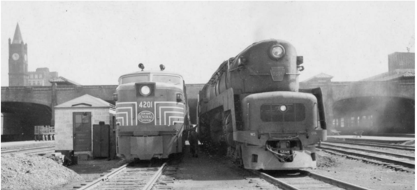
NYC DPA-2a 4201 (Alco PA-1) and PRR T-1 5504 line up on the west end of the Indianapolis Union Station train shed. NYCSHS PB531010
