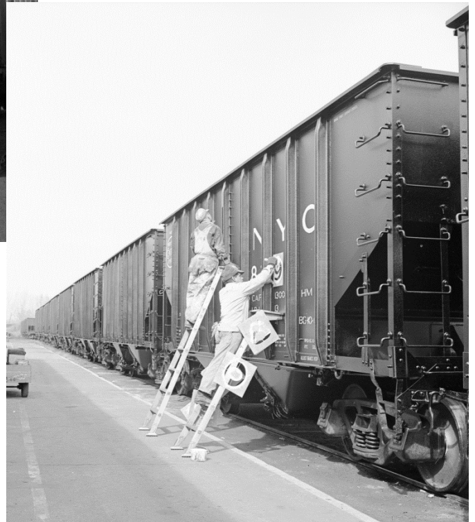
In the mid-1960s, Beech Grove crews converted 1948-1949 built offset-side, two-bay hoppers into Lot 942-H ribbed-sided hoppers. [NYCSHS NG525181 and NG525378]
