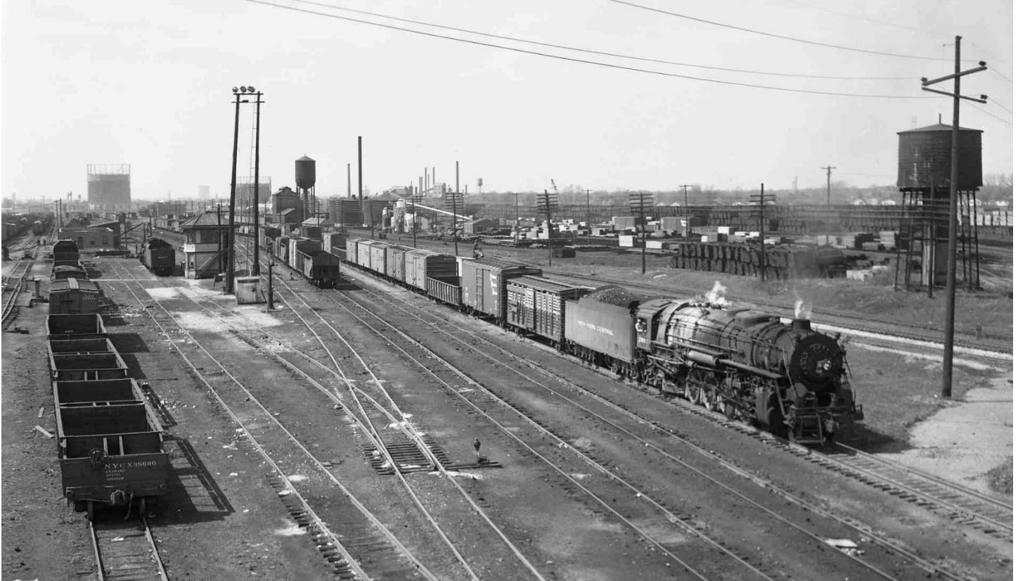
Kankakee-Indianapolis train KI-2 enters Middle Hill behind L-2c Mohawk No. 2802. The Indianapolis “skyline” in the distance is actually the large Prospect Street plant of Citizens Gas and Coke Utility. [Jeremy Taylor photo, NYCSHS NG503034]
