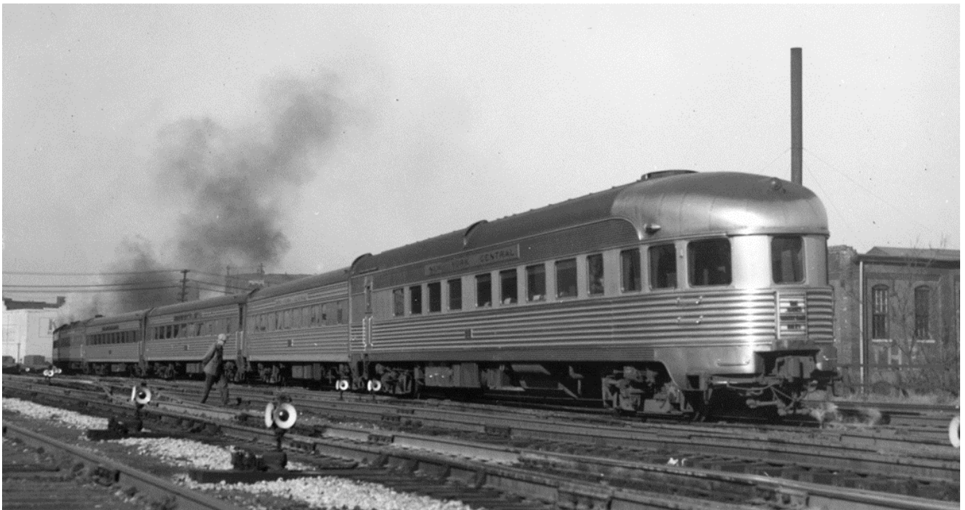
The postwar Riley featured an all-stainless steel consist – but with a mixture of Budd and Pullman-Standard coaches, Budd dining and tavern-lounge-observation cars, and baggage-coach combines built by American Car & Foundry. [Ed Nowak photo, NYCSHS PB574043]
