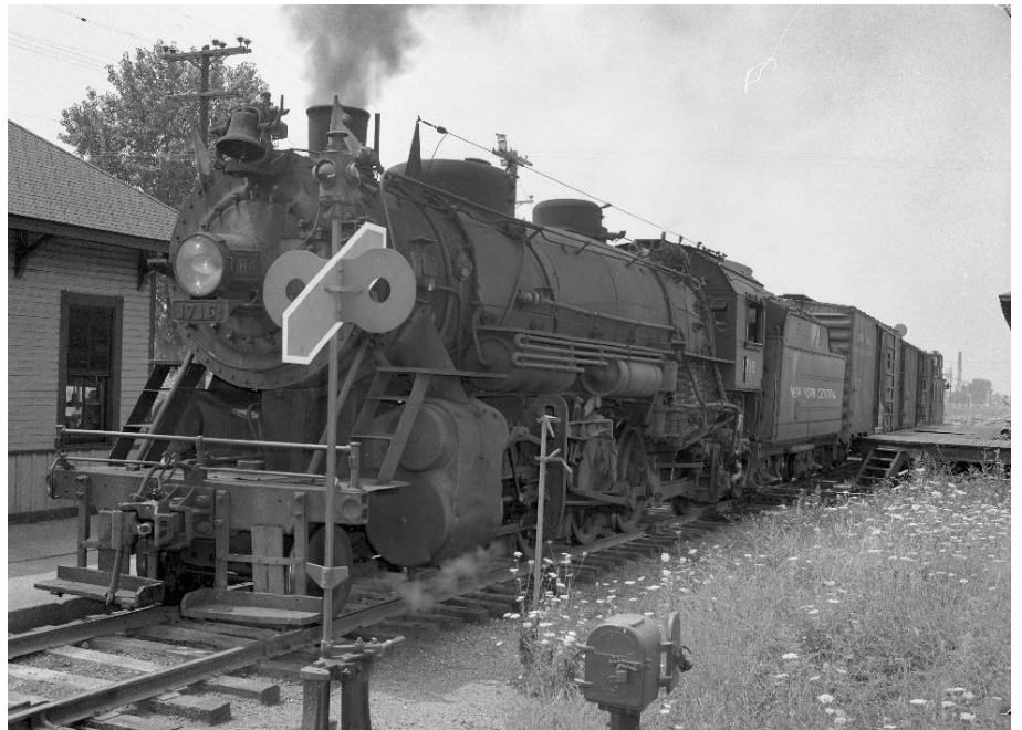
In 1948, H-6a No. 1716 was participating in a test of radio equipment at the Shirley depot (right). [NYCSHS WR410120]
