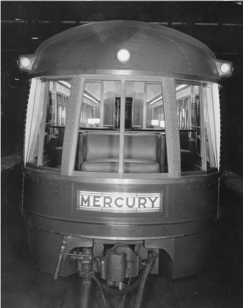
In 1936, the Beech Grove Shops transformed Henry Dreyfuss's drawing and 1927 coach into the Mercury's remarkable parlor-observation car. [NYCSHS WR240216 and PB602139]
