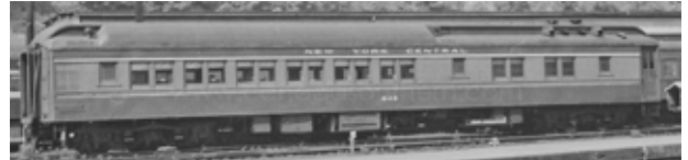
A rare aisle-side photo of #648. Roof detail shows a pair of blower vents and a pair of remaining Ward vents; the two large kitchen ventilators look to be a style different from either the kits or the gable style. The photo nicely illustrates the post-53 two-tone grey scheme. John S. Horvath Collection, Canada Southern Collection
