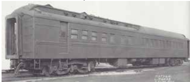
Pullman Company photo of #427 (later #638), taken after application of Pullman mechanical air-conditioning, 2/21/34. Note five-grab end ladder, gable-style range vents, long kitchen
