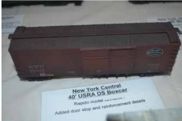
Rapido HO-scale NYC Lot 382-B 40'6" USRA double sheathed steel underframe boxcar 290173. The prototype was built by ACF in 1919. Modeled by Doc Snyder, who added door stop and reinforcement details to his model and marked his car as serviced in W. Springfield, Mass.
