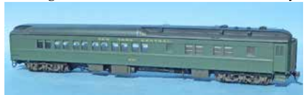
Completed model, aisle side; note prism windows, shades, and grab bars.
