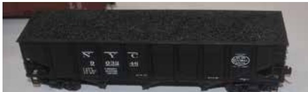
S-scale model of NYC Lot 588-H 38' 10" 3-bay all steel self-clearing hopper car 903246 built by Standard Steel Car Co. at Butler, Penna. in April 1920. The prototype was modified with panel sides at the NYC Avis, Penna. shop. Model by Jim Kindraka.
