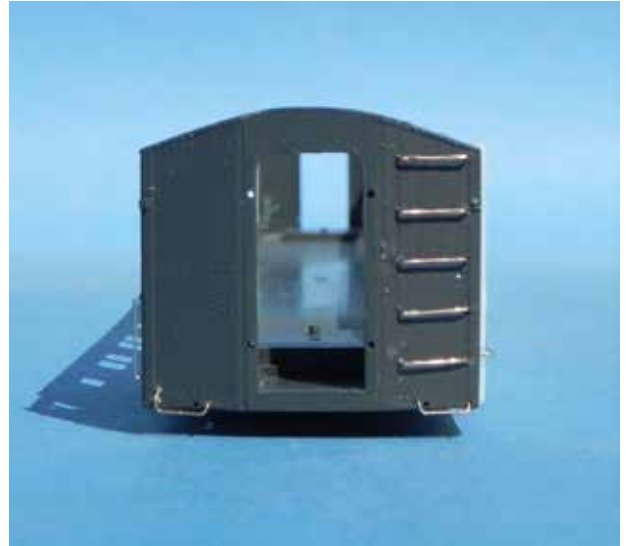
To match the prototype photo, a five-grab ladder (rather than six) was installed on the kitchen end.
