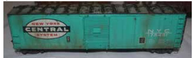
Stuart Thayer's HO-scale Proto 2000 model of NYC Lot 692-B 50' 6" all steel boxcar 176481 built by Despatch Shops, Inc. in February 1941. Although the car is still in full NYC markings, the "PGH 5-74" shop code indicates we are in the PC era.
