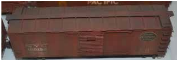
HO-scale model of NYC Lot 842-B 40' 6" all steel boxcar 180190 built by Pullman in Michigan City, Ind. in 1952. The shop code is hard to read through all that road grime but looks to be either Adrian, Mich., or the Ashtabula, Oh. old shop. Model by Chris Zygmunt.
