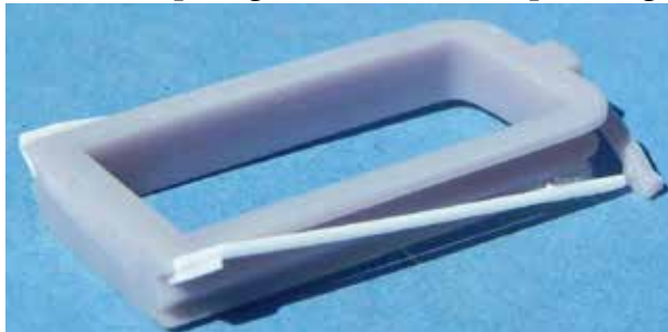
Rattle bars (styrene rod) are added to the diaphragms.
