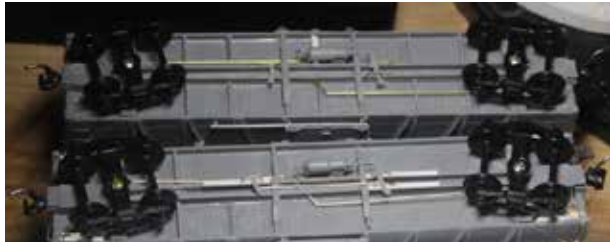
Under body details Note strips on middle and bottom cars Note styrene stirrup mounting members in corners.
