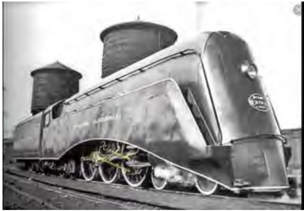
Steps were added to the pilot along with a handrail on the front. However, the hinges were removed, and bolts put back in. NYCSHS Collection.
