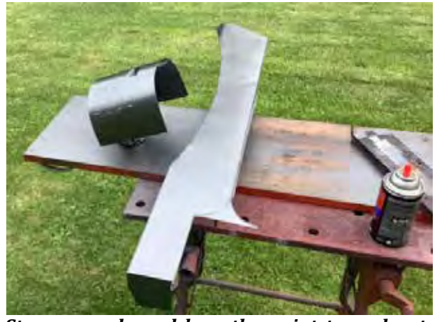
Steve was pleased how the paint turned out. Warming the can a bit in water seemed to help.
