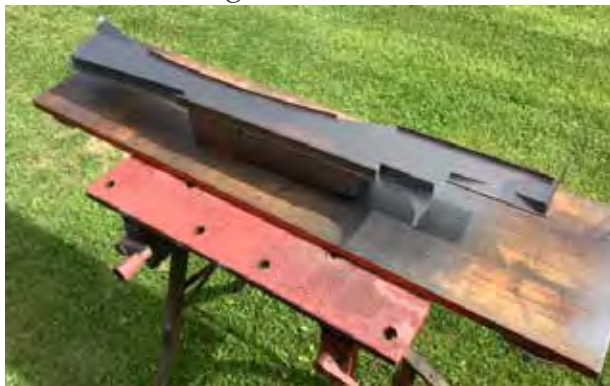
As mentioned, the backs were painted too to prevent rust.
