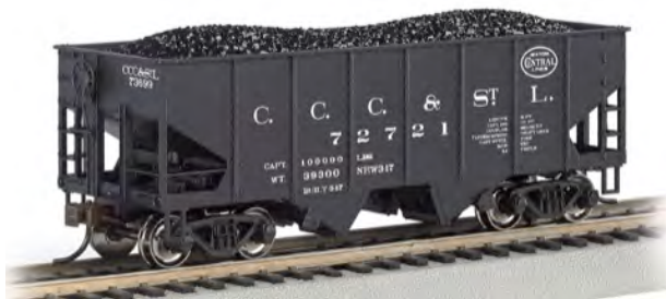
CCC&St.L 55-Ton Outside-Braced Hopper with removable coal load.
