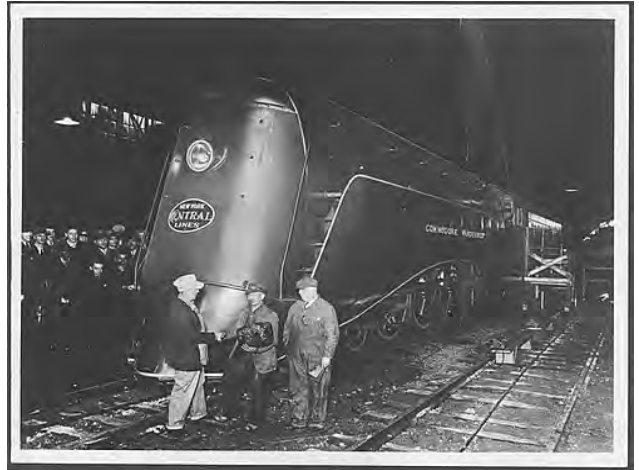
Right from West Albany. Notice the six bolts holding the door, no front rail or pilot steps. NYCSHS Collection.
