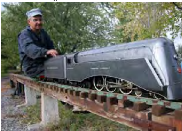
The original shroud as built with the dents and wrinkles beginning to show.
