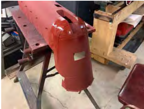
The nose got a few coats of sandable primer to make for a smoother contour. That was the plan anyway.
