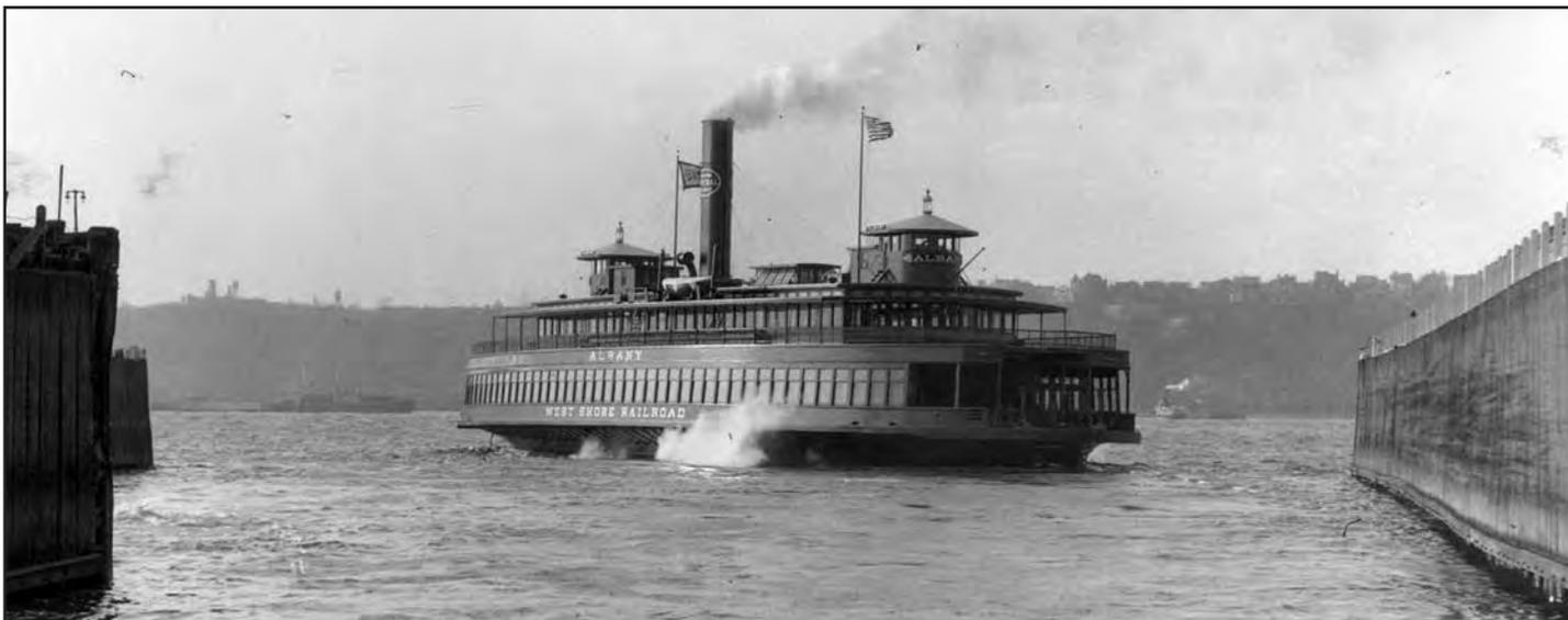
The *Albany* was the last ferry built for the West Shore Railroad, replacing the sole remaining sidewheel ferry, the *Buffalo*, in 1925. She was different in appearance from the West Shore's other ferries then in service, with pilot houses above the top deck and a different seating arrangement on the lower deck. Here she is at an early date in her career, leaving 42nd Street. NYC Neg. 9161, NYC SHS Collection.
